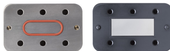
Figure 1: Ti inlet block used as active (working) electrode with sealing O-ring (left), rectangular Pt counter electrode in recess of black electrode holder (right)
